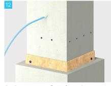
As the grout overflows from the upper grouting holes and the formwork holes in the corner of the couplers, close the holes using hose caps.
