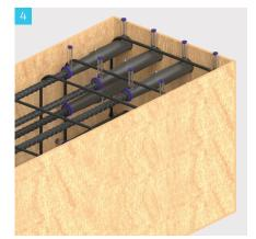
Attach the rest of the formwork. (Additional grouting hoses are necessary for mass grouting method).
