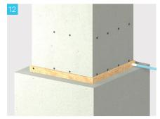
Attach the base formwork and start pumping the grout into the base.
