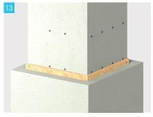
Once the grout overflows from the formwork hole, close both holes using a suitable method.
