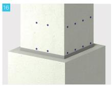
The braces may be removed 3 days after the completion of grouting.
