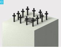
For individual coupler grouting method, insert the end seal onto the starter bar.
