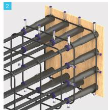
Install the clear hoses on the Ancon MGC-F Grout Couplers. Install the hose caps on all the clear hoses. Then, slide the grout couplers onto the position plug.
