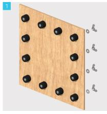
Install the position plugs onto the formwork. Secure using washer and wing nut, do not over tighten.
