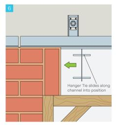
Insert Hanger Tie into the channel by turning head through 90° and slide the tie along the channel, pressing it into fresh mortar. Once in position, cover tie with more fresh mortar to create minimum 10mm vertical joint. Ensure the void between the underside of the support angle and the top of the hung brick is tightly packed with mortar.
