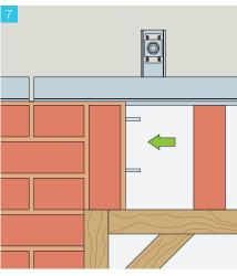
Push the next brick onto the dowelled Hanger Tie.
