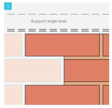
Build brickwork up to support angle level on each side of the opening, ensuring that the top three jamb bricks on one side of the opening are left out to allow the installation of the last soffit brick.
