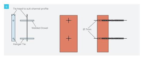
Offer up one brick and Hanger Tie to mark out dowel positions on the brick and remove. Drill two 7mm diameter holes through each brick at the dowel positions.
