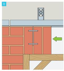
Cover the side of the brick with fresh mortar and position next brick.
