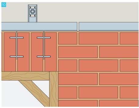
Install final jamb bricks, filling each joint with fresh mortar.
