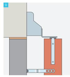
Repeat steps 6-8 until all soffit bricks are installed. Install Ancon SDB Restraint Ties as work progresses, typically at 450mm horizontal centres, ensuring that each tie is completely covered with mortar.
