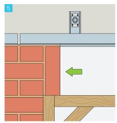
Install first soffit brick on to former, ensuring that the vertical joint to the adjacent brick panel is fully filled with mortar.
