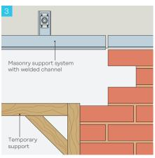
Install temporary support underneath the support angle on the line of the new soffit.
