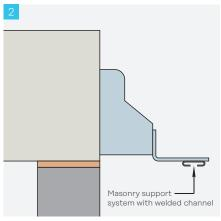
Install masonry support system in accordance with our installation guidance and drawings. The Hanger Tie system uses a support angle with a channel, normally Ancon 36/8, welded to the underside.
