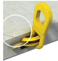
Clutch bearing crack
