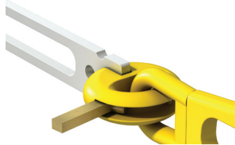
Conventional clutch has a round locking ring so the clutch is free to rotate around the anchor under shear load.
