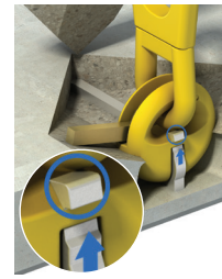
Complete rotation and failure
