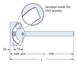
The cantilever is available in three standard lengths. Custom lengths are also available.
