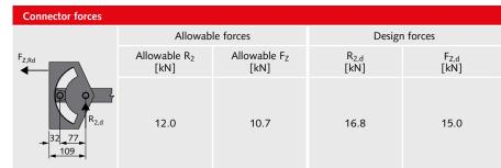
The values are adopted from the tables "maximum forces" and "connector reaction forces" normalization according  $f_{\rm y}.$
