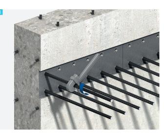
4 Slab reinforcement should be installed to the Engineer's details and the slab is cast to complete the application.
