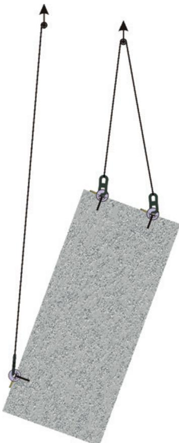
Turn the panel by transferring the load to the main hoist.
