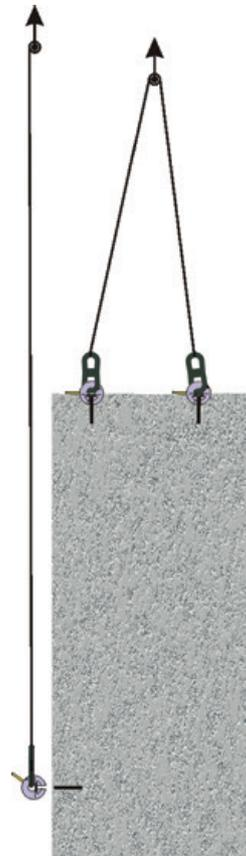
Remove the spin-up clutch. Hoist the panel into position and disconnect the top lift clutches, preferably with the aid of an elevated work platform or remote release when using the EdjPro remote release clutch.
