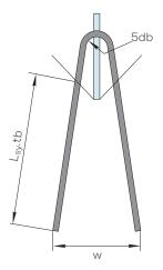
**Notes:** Locate the perimeter bar above the EdjPro anchor to control flexural cracking. N12 shear "w" bars may help control shear cracking at higher loads. Panel cracking and shear spalling is possible if the recommended loads are exceeded. Some anchor deflection is normal, particularly at high sling angles. For other panel thicknesses, please consult the Leviat technical team for design advice.
