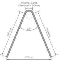
Recommended N16 Tension Bar Diagram 1
