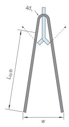
**Notes:** Locate the N16 perimeter "trimmer" bar above the EdjPro anchor to control flexural cracking. Shear "omega" bars may help control shear cracking at higher loads. Panel cracking and shear spalling is possible if the recommended loads are exceeded.
