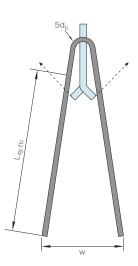
**Notes:** Locate the N16 perimeter "trimmer" bar above the EdjPro anchor to control flexural cracking. Shear "omega" bars may help control shear cracking at higher loads.
