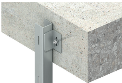
Top Connection of a WP3 Windpost to the Face of the Concrete
