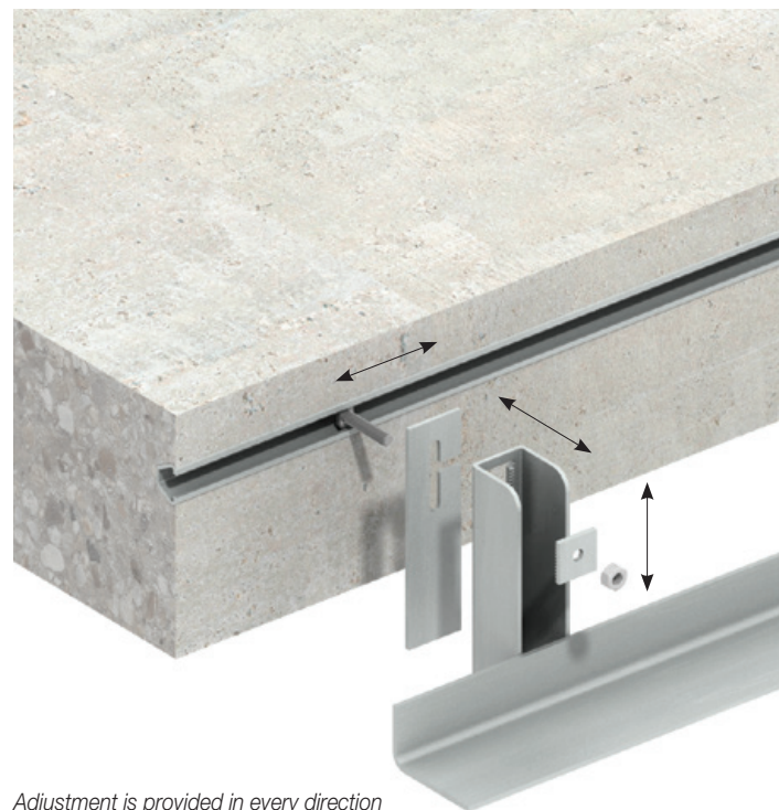
Adjustment is provided in every direction to allow for tolerance in the structural frame
