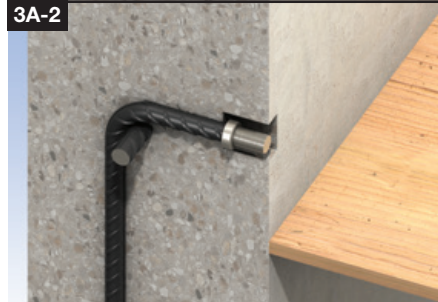
Remove the formwork and polystyrene and screw the locknut onto the fixed bar.
