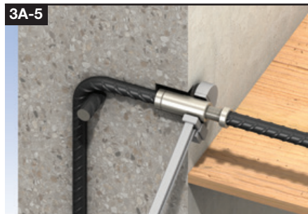
Screw the coupler from the continuation bar onto the fixed bar and lock tight with a wrench against the locknut.
