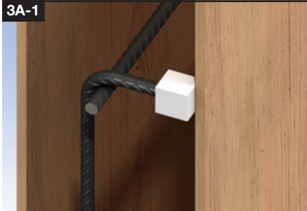
Place polystyrene foam with minimum dimensions as per table 2 below around the thread of the fixed bar with the C1 thread. Place the bar in position with the thread flush with the formwork and securely tie to the surrounding reinforcement.
