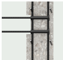
High performance KSN Anchor System. Bars are installed when required. No bending of bars. Less congestion in the wall.
