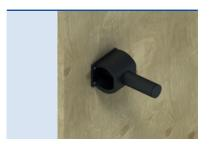
Nail the sleeve component to the shuttering ensuring that the sleeve is correctly orientated for the direction of the load. Check that the minimum spacing and edge distances are not exceeded. The label prevents debris from entering into the sleeve aperture and should not be removed. Fix all necessary reinforcement and pour the concrete.
