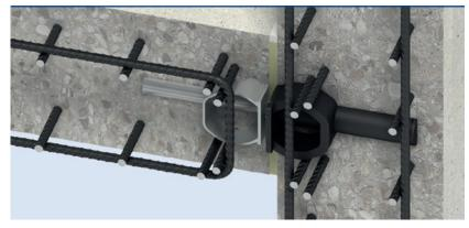
Fix the reinforcement around the dowel component and pour the concrete to complete the installation.
