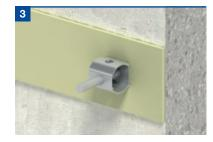
Position compressible joint filler of an appropriate width for applications where movement is expected between two sections of concrete. Push the dowel component through the joint filler until it is fully located in the sleeve component. It may be necessary to tap the dowel component to overcome the dimple which pinch holds the dowel in the sleeve and prevents dislocation when the concrete is vibrated.
