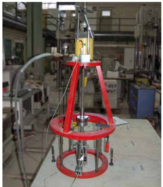
Test setup pull out tests
