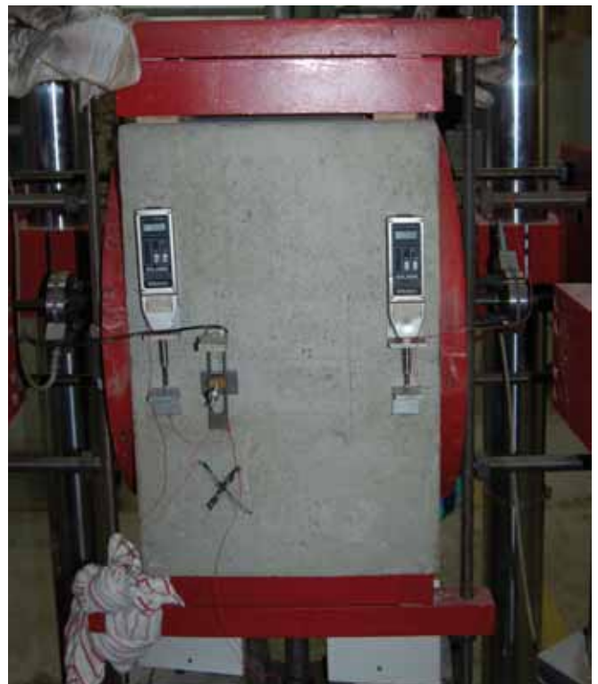
Test setup for cyclic load test
